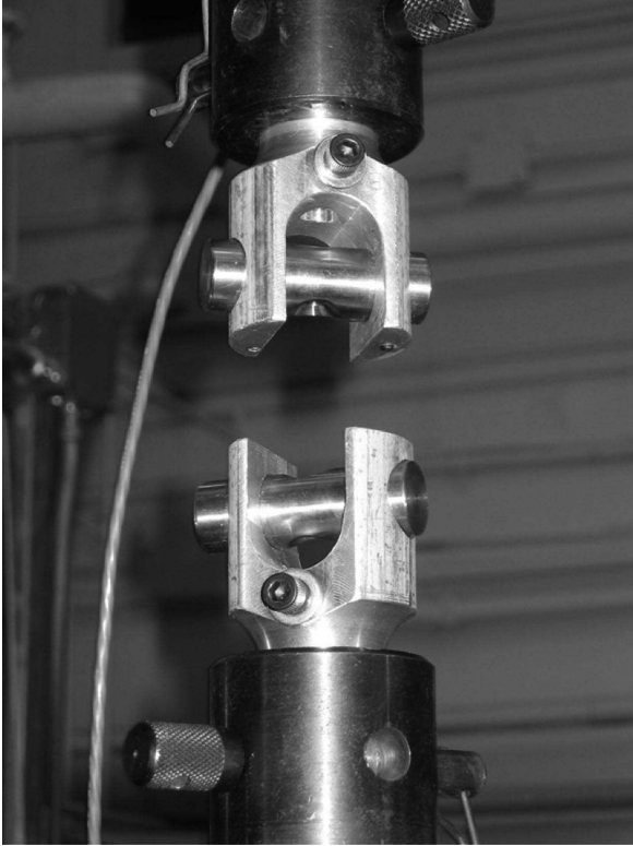
Fig. 2. Unique grips were designed to minimize tearing at the connection sites.
